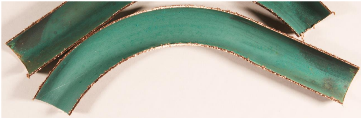
Fig. 4 Regular green carbonate patina formed on cold water pipes
