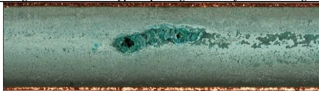
Fig. 10a – Case 7 Type 1 pitting -bore before cleaning
