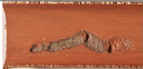
Fig. 11b – Case 30 Type 1 pitting – close up of pit
