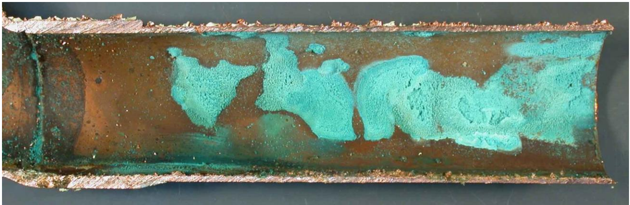
Fig. 3 Irregular phosphate-containing carbonate deposit on bore of cold water pipe
