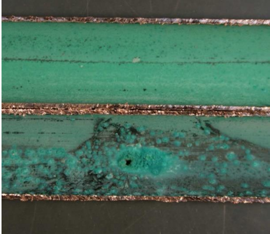
Fig. 14a – Case 10 MIC pitting -bore before cleaning
